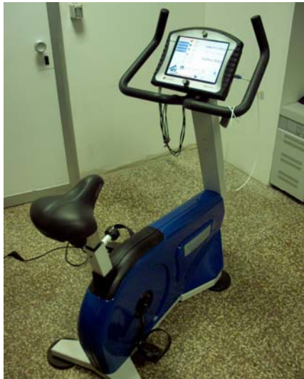
Figure 2: (a) Cyclette for cardiologic rehabilitation with ECG, pressure and oxymetry sensors. (b) Bike's software interface: signals are displayed in real time and parameters (heart rate, oxygen consumption and saturation, energy dissipation, exercise duration) are showed in the centre of the screen. A simple set of commands (Start, Connect, Parameters and Reset) allows to manage the rehabilitation session.
